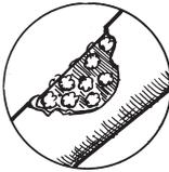
The mass is only effective as long as its structure is in sound condition. The mass can be damaged by blows to the cylinder or if the cylinder is dropped from height.
