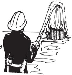
Once the fire is extinguished, continue to cool until the cylinders are no longer steaming. At this point approach the cylinders with caution, having tested the atmosphere with relevant safety instruments.
