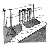
Since many cylinder gases are heavier than air, care must be taken to ensure any leaks cannot accumulate in ditches, drains or low lying areas.
